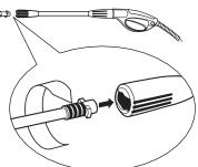
**Step 2** Insert the spray wand into the wand extension. Push in and turn clockwise to lock spray wand in place.
